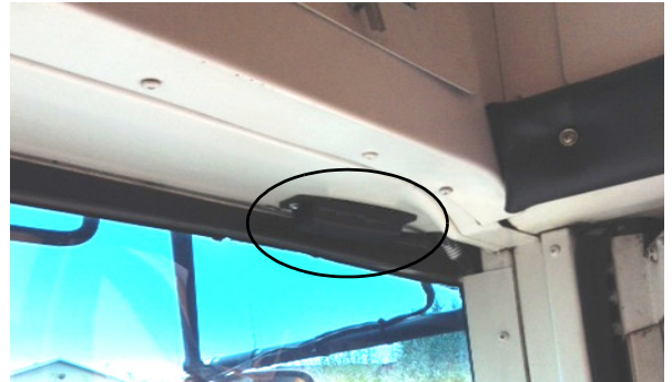
Inside fiberglass (NOT metal) wiring cabinet
