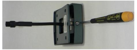
2. Position the back plate of the card reader on the vehicle surface and mark screw and center hole positions.
