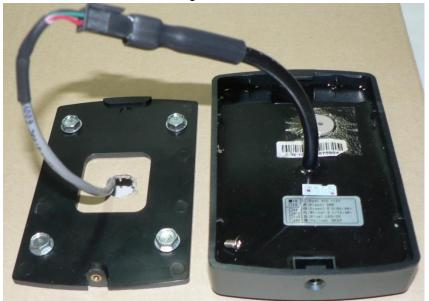
5. Thread the cable connector in the hole and reattach the card reader to the back plate.
