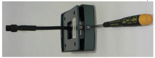
2. Position the back plate of the card reader on the vehicle surface and mark screw and center hole positions.
