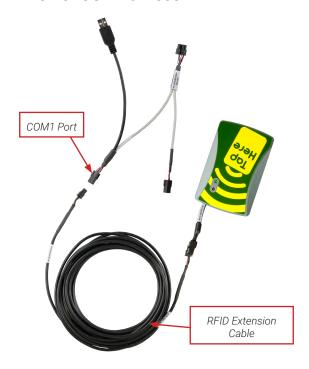
7. Connect the **RFID Power** and **USB** harness to the MDT.
