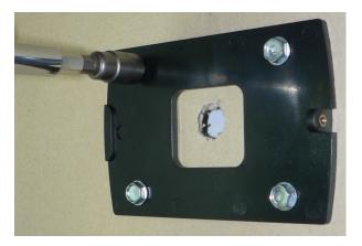
4. Run the RFID extension cable through the center hole and connect one end to the card reader (both ends are interchangeable).
