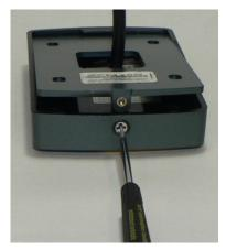
Position the back plate of the card reader on the vehicle surface, then mark the screw and center-hole positions.
