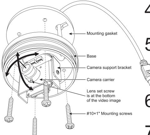
Use the four #10×1" mounting screws supplied with the camera to attach the camera to a wall or ceiling. Always put the mounting gasket between the base and the mounting surface.
