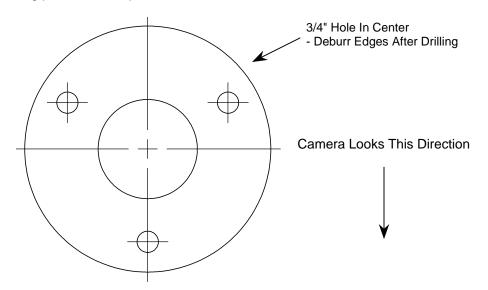
The bracket is attached to the mounting surface using the accompanying three pieces of 8-32x3/4" selfdrilling screws. Use a 5/16" socket to drive the screws into the sheet-metal mounting surface. The camera is then attached to the bracket using three pieces of 8-32x3/8" machine screws and 8-32 Nylock nuts included in your package. The camera harness runs up the center of the mounting post, providing a concealed cable run.
