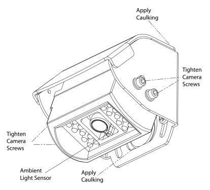
12 After the final alignment is complete, apply caulking along the top edge of the bracket, and caulk the cable hole if required.
