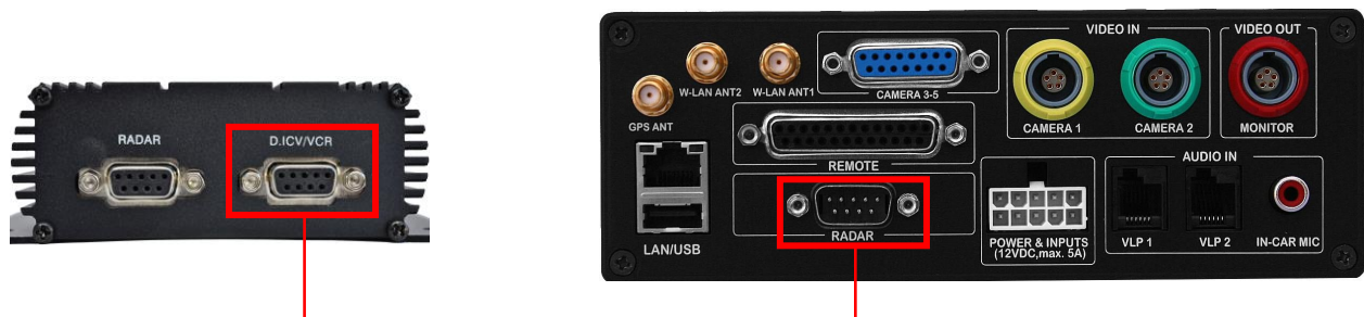
Figure 15: Connection from radar unit to DVR
