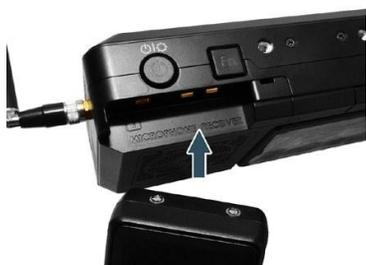
After the power is on, sync up your wireless microphone to your Fusion HD system. Hold the wireless microphone and use its two sync points at the bottom of the microphone transmitter to press against the first and third sync points (from the left) on your Fusion HD system. You will hear a beep from the microphone when it has successfully synced with your transmitter.
