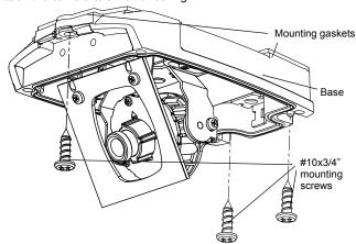
The mounting gaskets on the camera base seal the screw and cable holes when mounted on a flat surface.
