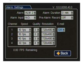
When these settings are complete, the camera will record at the lower setting selected in step 1 until the stop arm is deployed, which triggers Alarm 2 to set the camera recording settings to the levels set in step 3. When the stop arm closes the alarm is off and the cameras return to the settings in step 1. During playback in vMax View, multiple stop arm recordings will display as alarms on the Alarms tab. These stop arm alarms are not to be confused with driver alarms.
