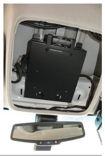
Install the monitor and loom the open area with  $\frac{3}{4}$  loom.
