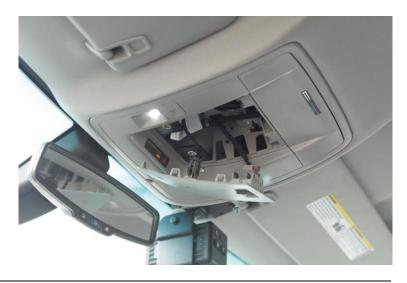
Remove the overhead control panel's (OCP) outer piece to gain access to the light switch and led connector. Remove the light switch and connector from the outer piece.
