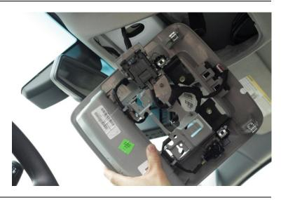
With the OCP removed, unclip the main OCP harness connector.
