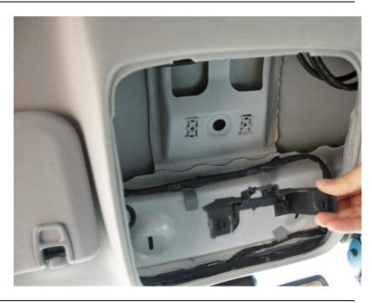
With the main harness detached from the OCP, install the airbag light module and light switch into the provided monitor bracket. Make sure the tabs from the light switch all clip in.
