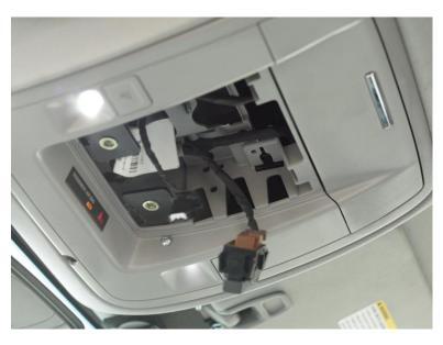
After removing the screws, carefully remove the entire overhead control panel.
