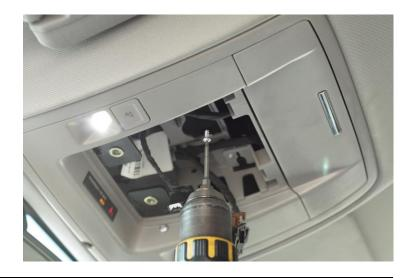
Remove the 2 T-10 torx screws which hold the overhead control panel in place.
