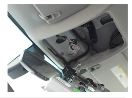
Carefully unclip all push tabs, airbag light module and led light connectors.
