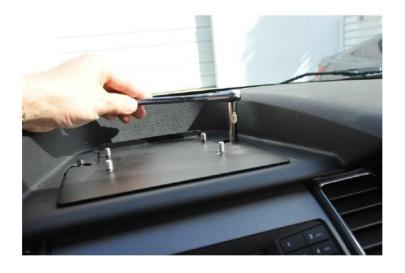
Align the monitor mount and secure with the (4) 7/16<sup>th</sup> locking nut provided.
