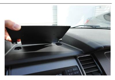
Secure adapter plate with existing 8mm bolts.
