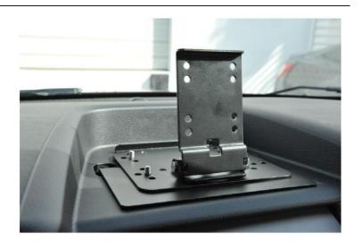
Use four (4) provided 10-32 x 3/8" Phillips pan head screws to secure the monitor mount to the back of the EDGE monitor.
