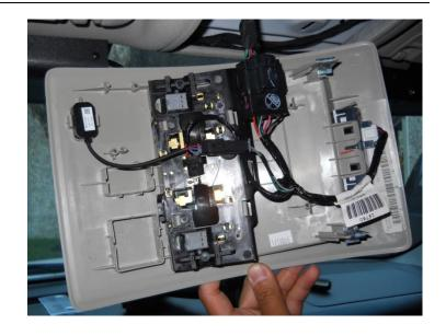
Remove the two (2) T15 Screws that hold the dome light compartment.
