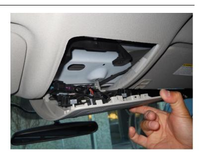
Disconnect all cables to the dome light except the passenger airbag light.
