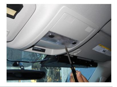
Remove the two (2) T15 screws to remove the overhead dome light.
