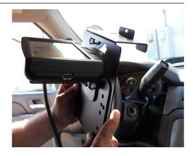
Secure the EDGE monitor mount to the Tahoe adapter plate using the four (4) provided 10-32 x 3/8" Philips pan head screws
