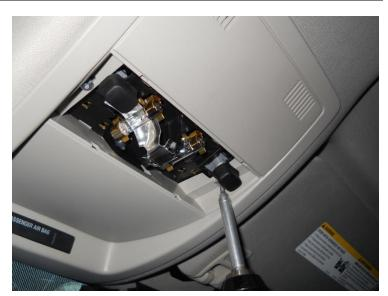
Pull down dome light from the side farthest away from the windshield to release the dome light.
