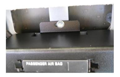
Secure the rest of the mount by using two (2) provided #10-16 x 1 1/4" self tapping screws to the round cutouts on the front of the mount.
