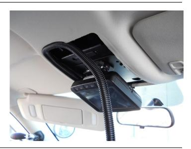
Make sure monitor can freely rotate and secure cables with zip ties.
