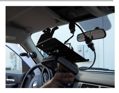
Secure the mount by using one (1) of the provided  $\#10-16 \times 1 \ 1/4$ " self tapping screws to the front of the mount.
