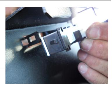
Make sure passenger airbag light is clipped in and secure.
