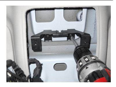
Use four (4) provided 10-32 x 3/8" philips pan head screws to secure the monitor mount to the back of the EDGE monitor.
