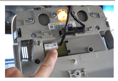
Remove the two (2) visor clips by removing the plastic tab on the back.
