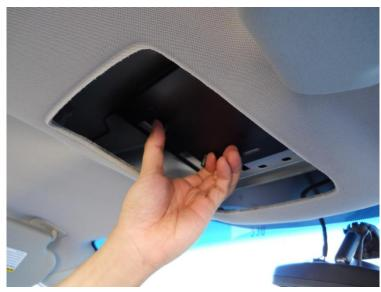
Secure the back part of the adapter plate by using the two (2) provided 7/16 locking hex screws.
