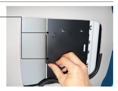
Secure the front of the adapter plate using one (1) provided 10-16 x 3/4" self tapping screws.
