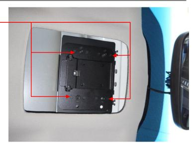
Use four (4) provided 10-32x 3/8" Philips pan head screws to secure the Edge monitor to the back of the monitor mount.
