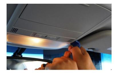
Disconnect the cable to the dome light
