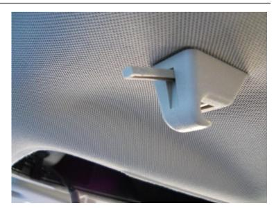
Remove the four (4) T20 Screws that hold the dome light compartment.
