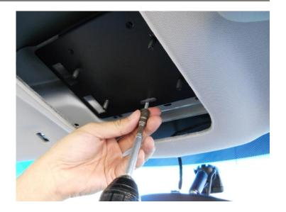
Secure the monitor mount with four (4) 1/4-20 hex nuts.
