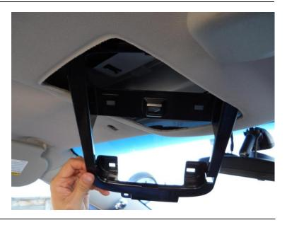
Slide in the Caprice adapter plate onto the roof crossbar of the vehicle.
